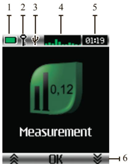
**Attention!** When the charge level is critically low and the device has switched off, malfunction or loss of measured data are possible and settings may be lost. Therefore, if the indicator is red, immediately connect the device to the charger or change the batteries.
